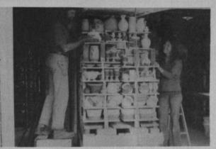
Wood kiln trolley almost stacked. Door pulled up by rope in foreground.
