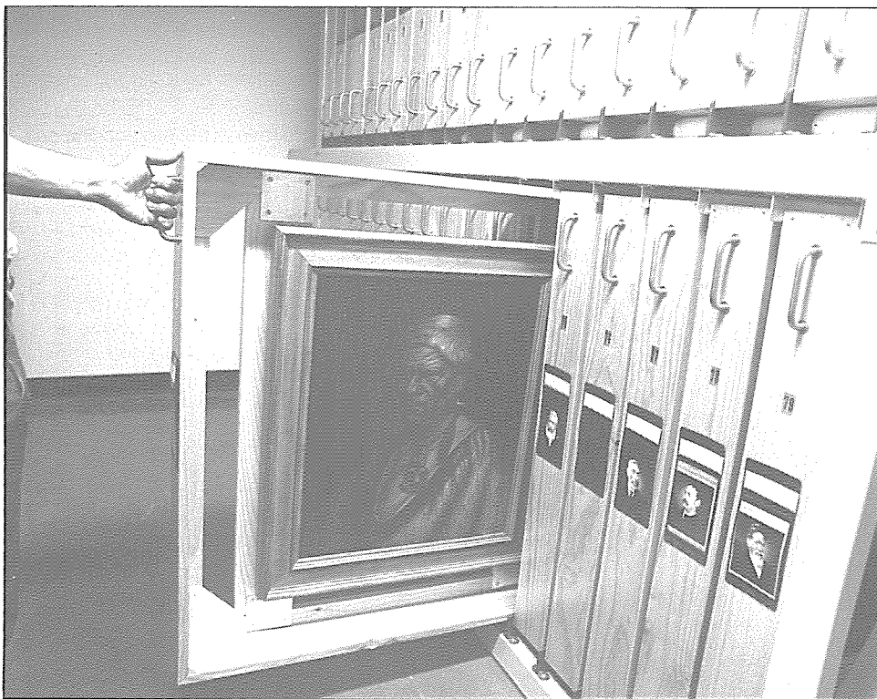
The ACAG developed box storage system with the box drawn out ready for removal.
