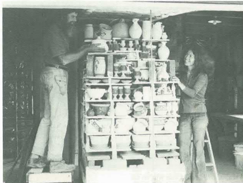
Wood kiln trolley stacked, door pulled up by rope. Wine jar and stand by John, goblets by Kathleen. Bowl 16 cm, and cheese dish 20 x 24 cm, all celadon glaze wax resist decoration.
