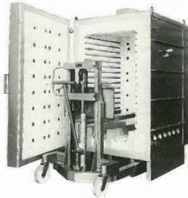
Fork lift loaded kilns
