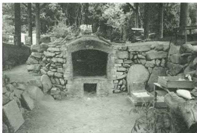
Tunnel kiln at the Nakazato Takashi workshop.
