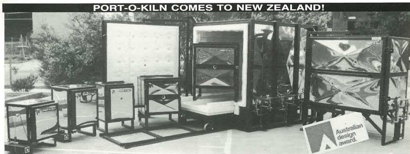
From left to right: China Painter; Model 2000 Ceramics Kiln; Chameleon (approx. 2 c.f. Stoneware Kiln) Model 40 (Stoneware); Model 80 (Stoneware); 72 c.f. trolley; 18 c.f. model.
