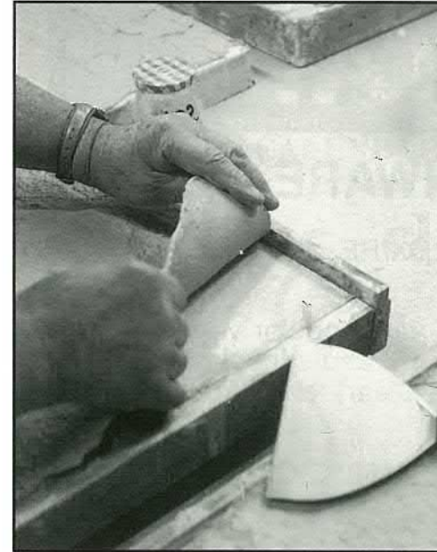
8: When stiffened, the slabs can be removed and stored between plastic sheets until needed.
