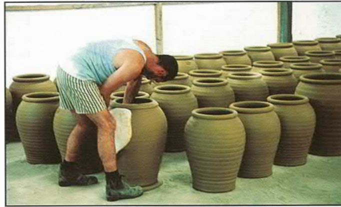
The greenware drying room
